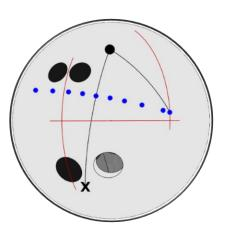
The "X" on the diagrams indicates the Preferred Spin Axis (PSA / Mass Bias) of the drilled ball, and the line that connects the PSA and PIN after drilling is referred to as the "Pin to Spin Line". The important feature of the "Pin to Spin Line" is that the ball revs up when the migrating axis crosses this line so the sooner the migrating axis crosses the "Pin to Spin Line", the sooner the ball rev up.
