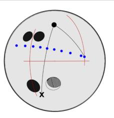
The "X" on the diagrams indicates the Preferred Spin Axis (PSA / Mass Bias) of the drilled ball, and the line that connects the PSA and PIN after drilling is referred to as the "Pin to Spin Line". The important feature of the "Pin to Spin Line" is that the ball revs up when the migrating axis crosses this line so the sooner the migrating axis crosses the "Pin to Spin Line", the sooner the ball revs up.
