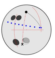
The "X" on the diagrams indicates the Preferred Spin Axis (PSA / Mass Bias) of the drilled ball, and the line that connects the PSA and PIN after drilling is referred to as the "Pin to Spin Line" is that the ball revs up when the migrating axis crosses this line so the sooner the migrating axis crosses the "Pin to Spin Line", the sooner the ball rev up.
