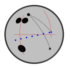
The "X" on the diagrams indicates the Preferred Spin Axis (PSA / Mass Bias) of the drilled ball, and the line that connects the PSA and PIN after drilling is referred to as the "Pin to Spin Line" is that the ball revs up when the migrating axis crosses this line so the sooner the migrating axis crosses the "Pin to Spin Line", the sooner the ball rev up.
