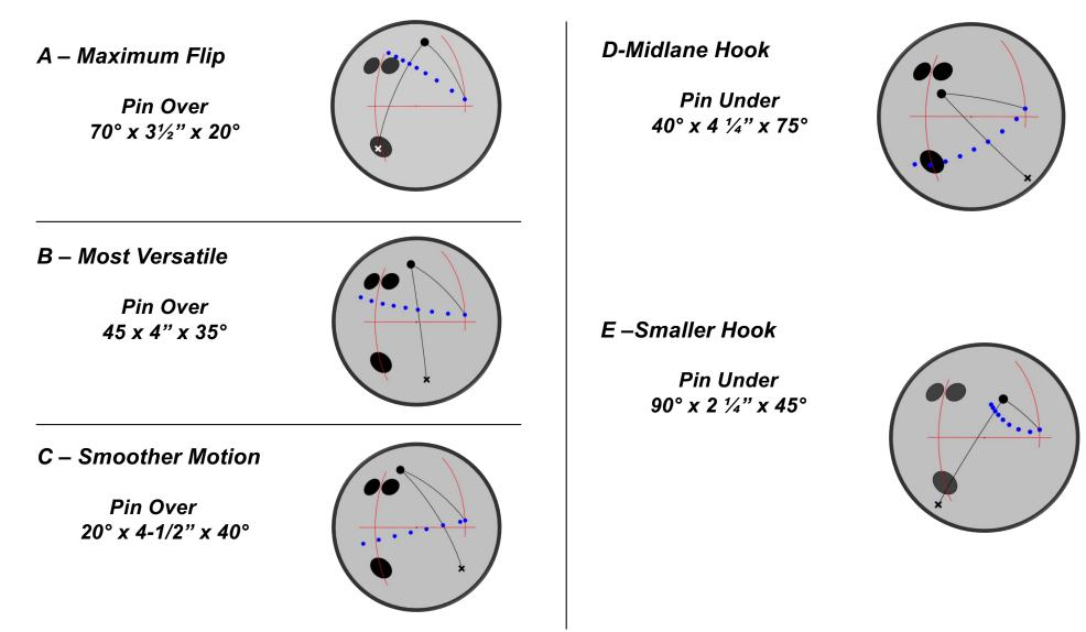
The "X" on the diagrams indicates the Preferred Spin Axis (PSA / Mass Bias) of the drilled ball, and the line that connects the PSA and PIN after drilling is referred to as the "Pin to Spin Line". The important feature of the "Pin to Spin Line" is that the ball revs up when the migrating axis crosses this line so the sooner the migrating axis crosses the "Pin to Spin Line", the sooner the ball rev up.
