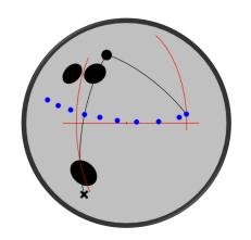
The "X" on the diagrams indicates the Preferred Spin Axis (PSA / Mass Bias) of the drilled ball, and the line that connects the PSA and PIN after drilling is referred to as the "Pin to Spin Line". The important feature of the "Pin to Spin Line" is that the ball revs up when the migrating axis crosses this line so the sooner the migrating axis crosses the "Pin to Spin Line", the sooner the ball rev up.
