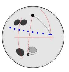
The "X" on the diagrams indicates the Preferred Spin Axis (PSA / Mass Bias) of the drilled ball, and the line that connects the PSA and PIN after drilling is referred to as the "Pin to Spin Line". The important feature of the "Pin to Spin Line" is that the ball revs up when the migrating axis crosses this line so the sooner the migrating axis crosses the "Pin to Spin Line", the sooner the ball rev up.
