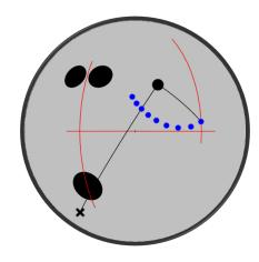
The "X" on the diagrams indicates the Preferred Spin Axis (PSA / Mass Bias) of the drilled ball, and the line that connects the PSA and PIN after drilling is referred to as the "Pin to Spin Line". The important feature of the "Pin to Spin Line" is that the ball revs up when the migrating axis crosses this line so the sooner the migrating axis crosses the "Pin to Spin Line".
