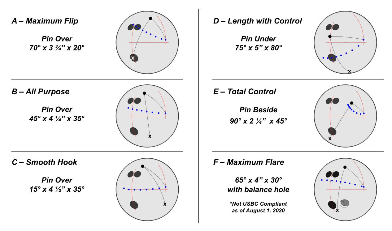
The "X" on the diagrams indicates the Preferred Spin Axis (PSA / Mass Bias) of the drilled ball, and the line that connects the PSA and PIN after drilling is referred to as the "Pin to Spin Line". The important feature of the "Pin to Spin Line" is that the ball revs up when the migrating axis crosses this line so the sooner the migrating axis crosses the "Pin to Spin Line", the sooner the ball revs up.
